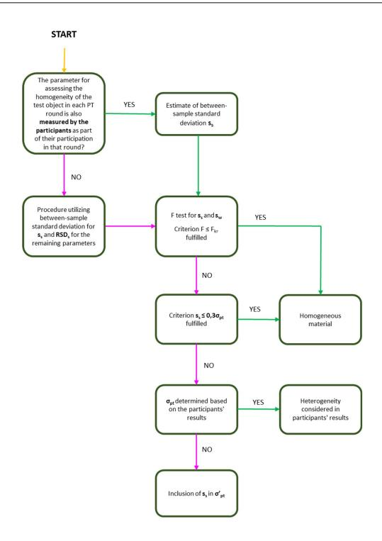
Fig. 1. Homogeneity assessment algorithm in proficiency testing
